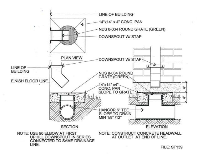
UNDERGROUND DRAINAGE AT DOWNSPOUTS SCALE: 1" = 1'-0"
